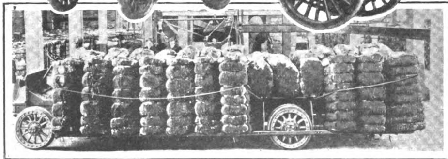
Upper—The modern way of collecting garbage. The low frame allows easy loading Middle—Five-ton electric street cleaning tractor made by the General Vehicle company for use in New York City Lower—Six-ton electric built especially for moving cotton. Loading is facilitated by the underslung frame
